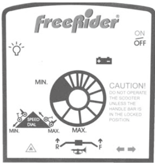
Control console label
